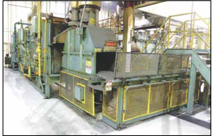
AFC-HOLCROFT HX0749 BATCH FURNACE HEAT TREAT FURNACE SYSTEM
